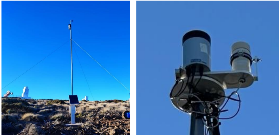
Figure A.10. Left panel: the ASTRI ARRAY meteo station close to the ASTRI-2 telescope. Right panel: the All Sky Camera together with the Sky Quality Monitor.
